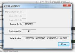
If the communication is working it is possible to proceed with the firmware update. Click on "close" on the "Device Signature" window. In the Flash Magic main window, click on "Start" to begin the programming. Wait until the end of the process, then turn off and on the FDM-DUO.
